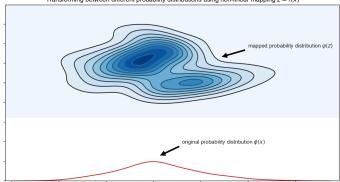
Transforming between different probability distributions using non-linear mapping z = f(x)
