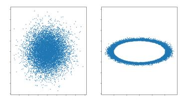
Using  $\phi(x) = (\frac{x}{|x|} + \epsilon * x)$  to transform random Gaussian noise to a Torus
